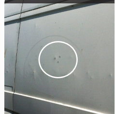
Outward dents to panel
